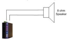
• Two 8 Ohm speakers must be wired in series
